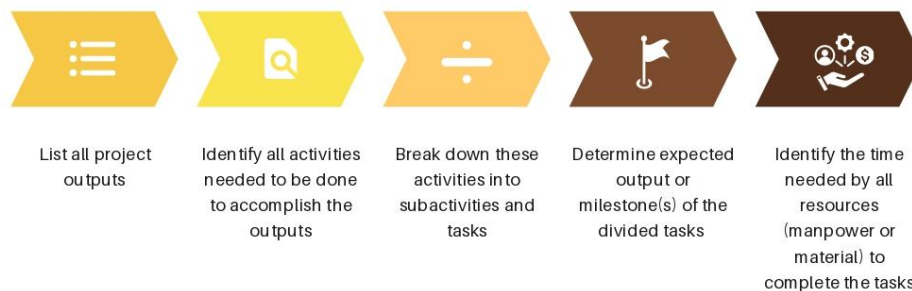
Figure 3: Development steps of a Work Breakdown Structure
