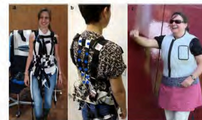
Fig. 2. The vibrotactile vest: adjustable harness (a) front and (b) back and (c) outer shell and skirt apron.
