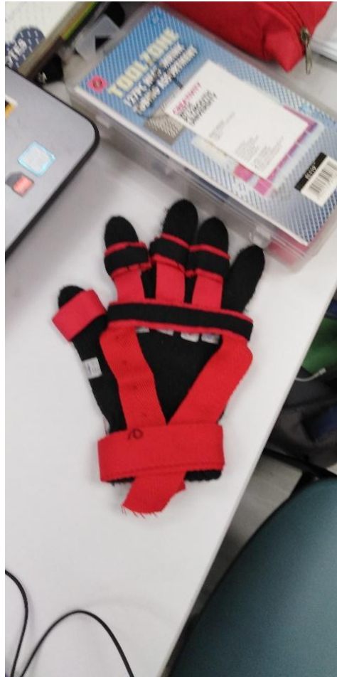
(Fig 4. The second prototype made from cotton tape and was manually sewn by hand.)
