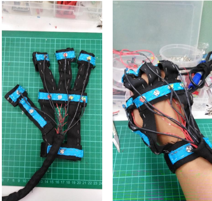
(Fig 11. The wires are banded together)
