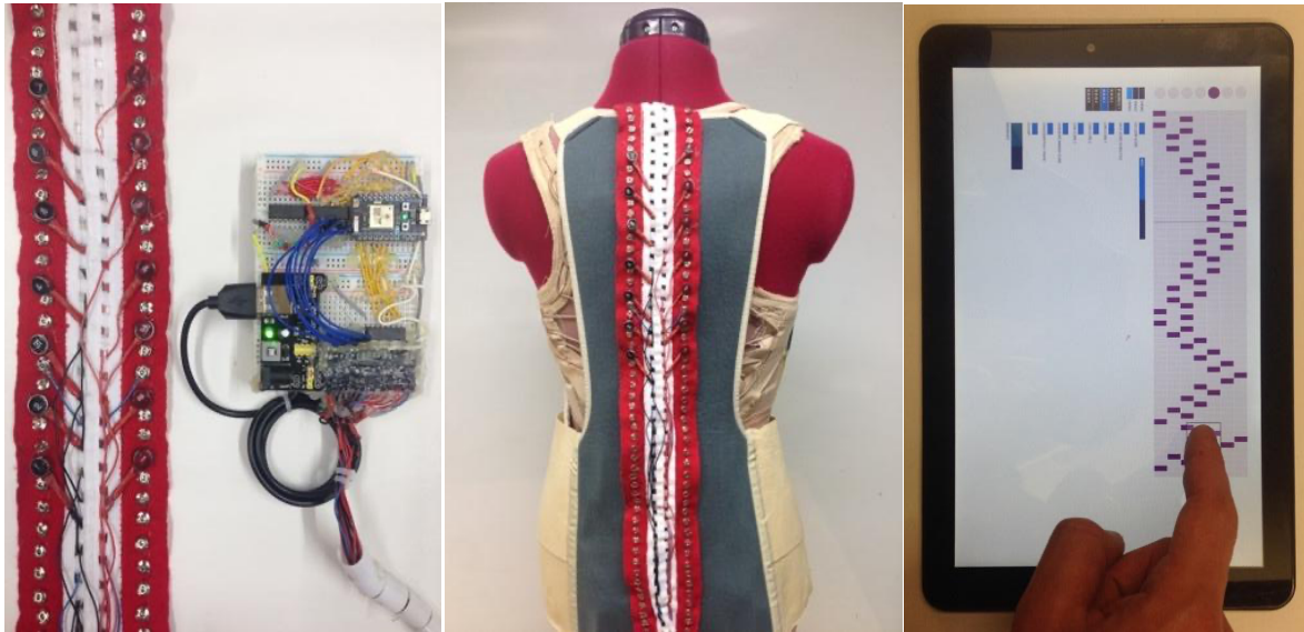
Fig. 2. From left to right: a) Close-up of repositionable motors and the microcontroller system and battery pack; b) The motors attached to a commercial posture correction vest; c) The mobile interface for programming the motors.
