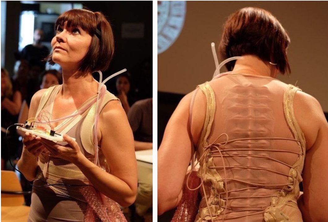
Fig. 5. Haplós used in Bisensorial, an award-winning proof-of-concept for a wearable neuroadaptive vibroacoustic therapy. Readings from a portable EEG sensor are used to create and evolve patterns of sound and vibration down the wearer's back to bring them to a desired mental state.
