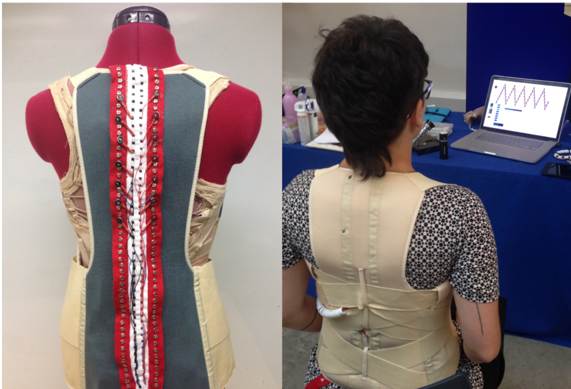
Fig. 1. Current prototype of the Haplós system attached to a commercially available back support garment and worn by a user. While the motors are stimulating this user's back, they can be applied to any part of the body.
