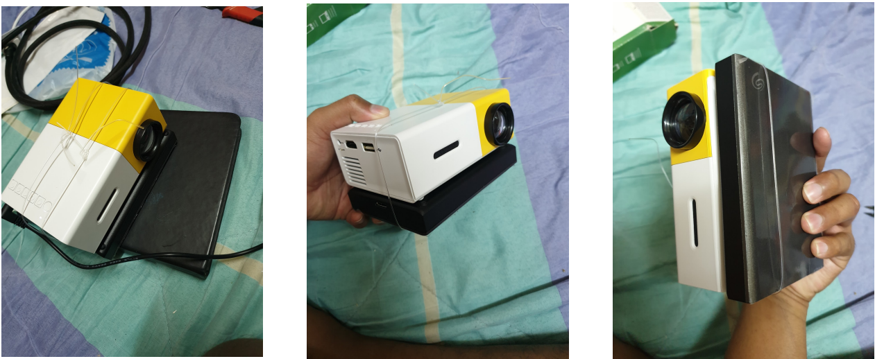
Plate 8, 9, 10. The projector and hard drive is attached together to save space inside the lantern.
