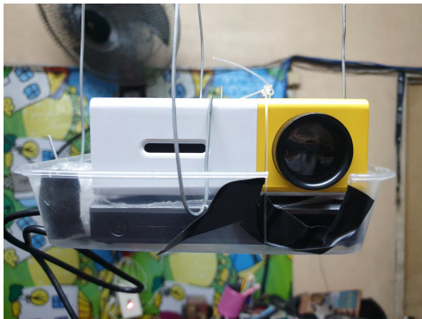
Plate 20, 21, 22, 23. The final version of the projector rigging.
