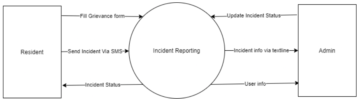
Figure 9. Incident Reporting Data Flow Diagram
