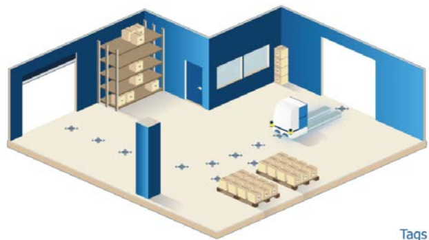
Figure 4: Tag following navigation
