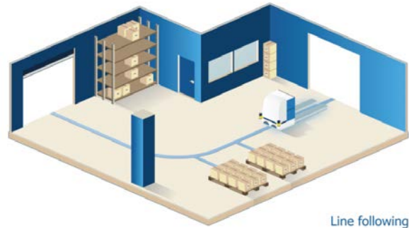
Figure 3: Line following navigation
