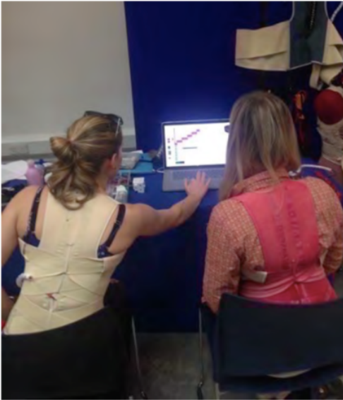
Figure 3: Two participants wearing back-support garments enhanced with Haplós. They are co-creating vibrotactile patterns and experiencing them simultaneously.
